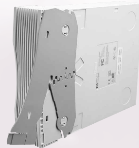
Rack-ready devices contain an ejection-lever assembly to assist in inserting the module into the rack enclosure and locking the module in place.
